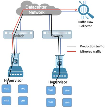
Figure 3: Pensando's Dynamic Flow Mirroring Solution
