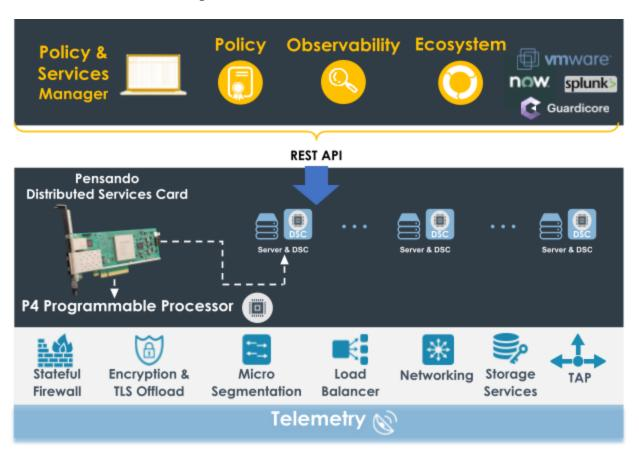
Since function accelerators like the **Pensando Distributed Services Card (DSC)** are securely separated from the host operating system and hypervisor, they are protected from attacks based on malware or rogue root admin access. Regardless of what happens in the application layer, infrastructure services are isolated, protected, and unable to be compromised.
